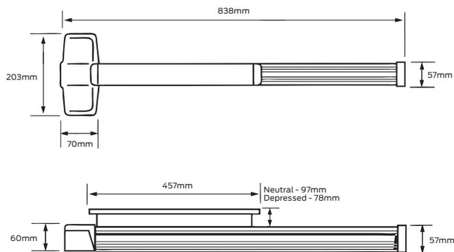
Device centre line to finished floor: 1011mm
