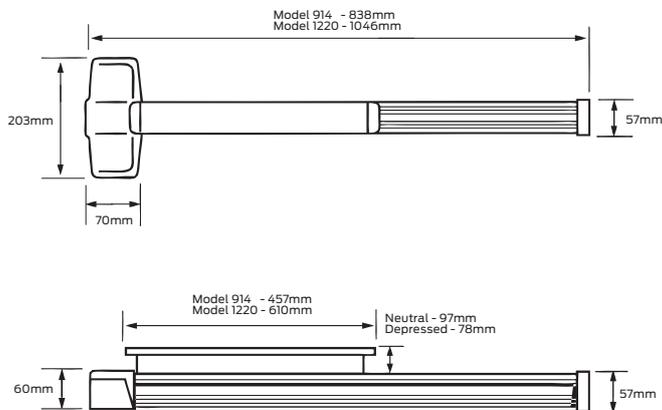
Device centre line to finished floor: 1011mm
