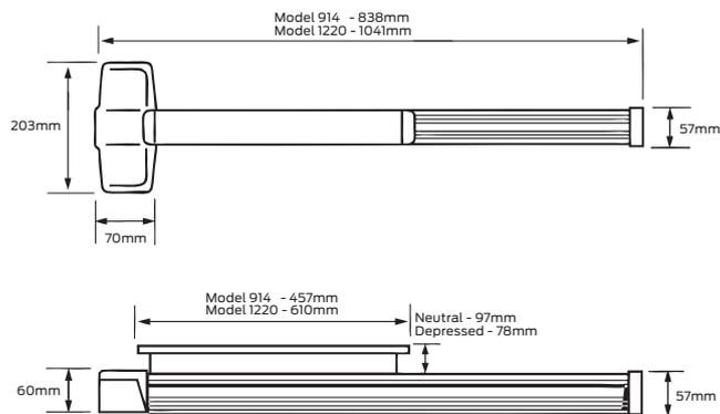
Device centre line to finished floor: 1011mm
