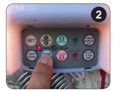
Press and hold the 'Door Code' button on the reciever board. Continue holding through steps 3, 4 & 5.
