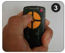
Press and hold a transmitter button on your new remote for 2 seconds.
