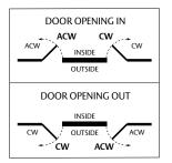
CW Left Hand open in (Clockwise) Right Hand open out
