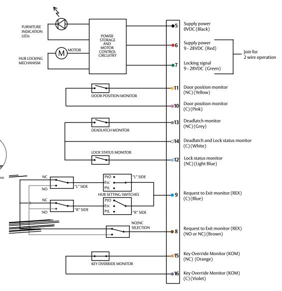
**SUPPLY POWER** ~ 300mA MAX (5 seconds), 20mA continuous if LEDs are activated
