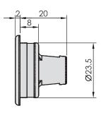
360RKSS Masonry Keeper - Cast 316 Stainless Steel - in Satin or Polished Stainless. For Windows Servery applications closing on Stone Kitchen Bench Tops.
