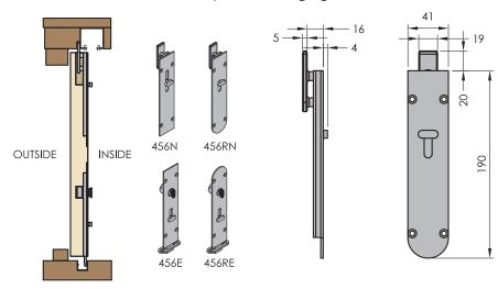
456REI Flush Bolts for flush floor timber panels.
