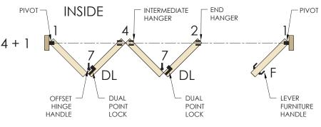
$\bigstar$  Two Set 2s mounted left and right are replaced with a single Set 8 if panels are rebated.
