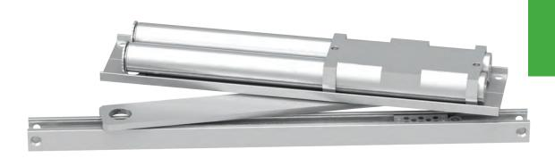
The concealed 6030 Series PACER® is a heavy duty, double acting closer designed to fit in a narrow, minimum 1-3/4" header. The single lever arm and roller assembly provides smooth, quiet door control and the choice of finishes and track functions meet virtually all architectural requirements. Installation at left illustrated with center pivot set (not included).
