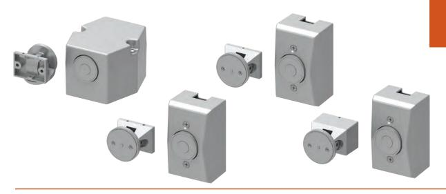
The Sentronic® SEM 7800 Series are heavy duty, electrically controlled door holding magnets. Magnets are fail safe and hold until the current is interrupted. A manual door closer is used to control and close the door. A choice of floor, recessed wall, or surface mounted wall magnets are available.
