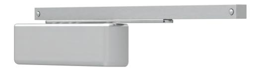
The 4040SE SENTRONIC® is a heavy duty, non-handed, nonsized closer/holder designed to provide single point hold-open for fire and smoke barrier doors. The door is held open until current interruption releases the holding mechanism and the door closes. Single lever (track) arm closer is specifically designed for interior doors. Choice of finishes, track functions, and installation accessories meet virtually all life safety requirements.
