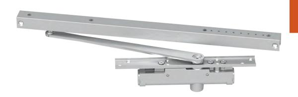
The 3130SE SENTRONIC® is a concealed in the door, closer/holder designed to provide single point hold-open for fire and smoke barrier doors. Door is held open until current interruption releases the holding mechanism and the door closes. Single lever (track) arm closer is specifically designed for interior doors.
