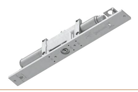
The 2310ME SENTRONIC® is a concealed heavy duty, electrically controlled closer/holder designed to provide infinitely adjustable hold-open for fire and smoke barrier doors. Door is held open until current interruption releases mechanism and the door closes. Single lever (track) arm closer is specifically designed for interior doors. Choice of finishes, cylinder functions, and installation accessories meet virtually all life safety requirements.
