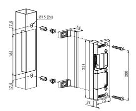
Electric strike for swing gates. The strike is equipped with a blocking system that withstands 500 kg pulling force. The deadbolt receiver has been reinforced with stainless steel. This innovation makes the strike even more robust. This keep is extremely strong and the ideal solution for all your access control. SE is available in two versions: E (Emissa - Fail Close)
